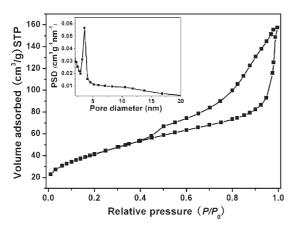
Figure 4. Nitrogen adsorption-desorption isotherm and (inset) the corresponding pore size distribution of the hierarchically porous  $Ce_{0.9}Sn_{0.1}O_2$  material calcined at 400 °C.
