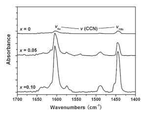
**Figure 6.** FTIR spectra of pyridine adsorption for the materials  $Ce_{1-x}Sn_xO_2$  (x = 0-0.10) at a deposition temperature of 200 °C.
