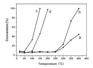
**Figure 7.** CO conversion as a function of temperature for the as-prepared CeO<sub>2</sub> (line a), hierarchical macrocellular/mesoporous Ce<sub>0.9</sub>Sn<sub>0.1</sub>O<sub>2</sub> (line b), Pt/macro-/meso-Ce<sub>0.9</sub>Sn<sub>0.1</sub>O<sub>2</sub> catalyst (line c), and Pt/meso-Ce<sub>0.9</sub>Sn<sub>0.1</sub>O<sub>2</sub> catalyst (line d).
