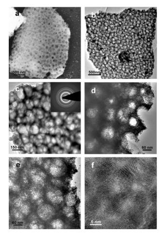
Figure 3. a) Representative SEM image, b,c) typical TEM images, and d–f) high-magnification TEM images of the hierarchically macrocellular/mesoporous Ce<sub>0.9</sub>Sn<sub>0.1</sub>O<sub>2</sub> materials calcined at 400 °C. The inset in (c) is the corresponding SAED pattern.
