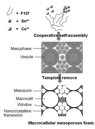
**Figure 5.** Possible mechanistic scheme for the formation of the hierarchically macrocellular/mesoporous foamlike cerium–tin mixed oxide with nanocrystalline framework by using a triblock copolymer as single template.
