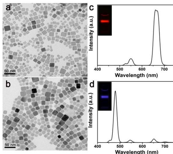
**Figure 1.** TEM images of a) NaYF<sub>4</sub>: Yb, Er/Mn UCNPs and b) NaYF<sub>4</sub>: Yb, Tm UCNPs. Upconversion luminescence spectra of c) NaYF<sub>4</sub>: Yb, Er/Mn UCNPs and d) NaYF<sub>4</sub>: Yb, Tm UCNPs. Inset: visible luminescence photograph of UCNPs using 980 nm excitation intensity of 0.5 W/cm<sup>2</sup>.
