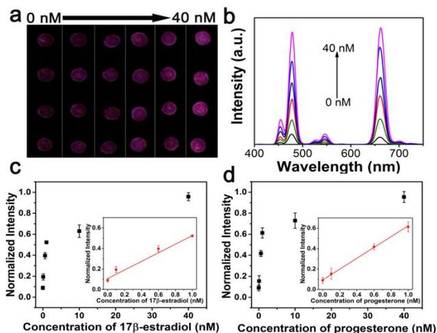
**Figure 5.** a) Luminescence photograph of the biosensor upon the addition of various concentrations of 17 $\beta$ -estradiol and progesterone in buffer solution. b) The luminescence spectra of the biosensor with various concentrations (0, 0.1, 0.6, 1, 10 and 40 nM) of 17 $\beta$ -estradiol and progesterone using 980 nm excitation intensity of 0.5 W/cm<sup>2</sup>. Standard curve of upconversion luminescence intensity versus the concentration of c) 17 $\beta$ -estradiol and d) progesterone.
