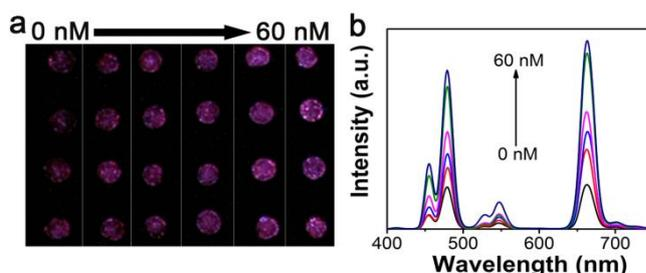
**Figure 6.** a) Luminescence photograph of the biosensor upon the addition of various concentrations (0, 0.6, 1, 10, 40 and 60 nM) in serum. b) The luminescence spectra of the PC microchip with various concentrations (0, 0.6, 1, 10, 40 and 60 nM) of 17 $\beta$ -estradiol and progesterone using 980 nm excitation intensity of 0.5 W/cm<sup>2</sup>.
