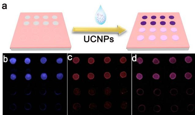
**Figure 3.** a) Schematic representation for the immobilization of UCNPs on the fabricated substrate. Luminescence images of the PC substrate after the deposition of b)  $\text{NaYF}_4: \text{Yb, Tm}$  UCNPs, c)  $\text{NaYF}_4: \text{Yb, Er/Mn}$  UCNPs and d) both kinds of UCNPs with 980 nm illumination intensity of  $0.5 \text{ W/cm}^2$ .
