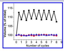
Figure 4. Reversible swelling and shrinking of light-responsive dynamic hydrogels in response to alternate irradiation by UV and visible light. Black curve: dynamic hydrogel containing cDNAs with azobenzene modification. Blue curve: control hydrogel (C1) containing cDNAs without azobenzene modification;. Red curve: control hydrogel (C2) containing noncDNAs with azobenzene modification.
