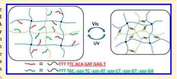
Specifically, a dynamic hydrogel was prepared by grafting azobenzene-tethered ssDNA and its cDNA to the hydrogel network. The macroscopic volume of the hydrogel can be manipulated through the photoreversible DNA hybridization controlled by alternate irradiation of UV and visible light. The effects of synthetic parameters including the concentration of DNA, polymer monomer, and permanent cross-linker are also discussed.
